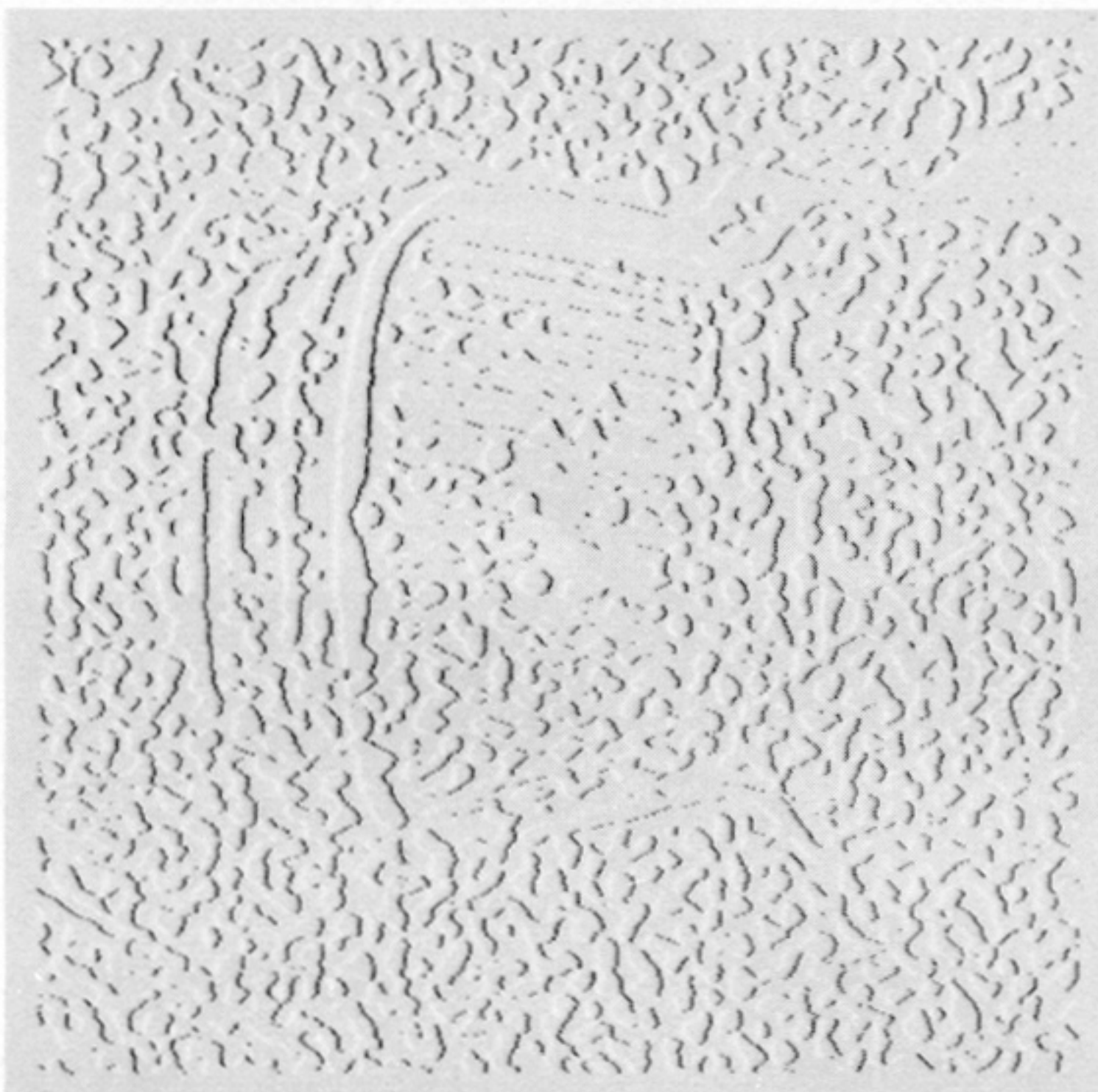
FIGURE 5. Examples of zero crossings. A natural image is indicated in (a). Below are examples of the zero crossings, obtained from different-sized \nabla^2 G operators, with central panel widths of (a) 36, (b) 18, (c) nine and (d) four picture elements. The positive zero crossings are shown as white, the negative ones as black.
